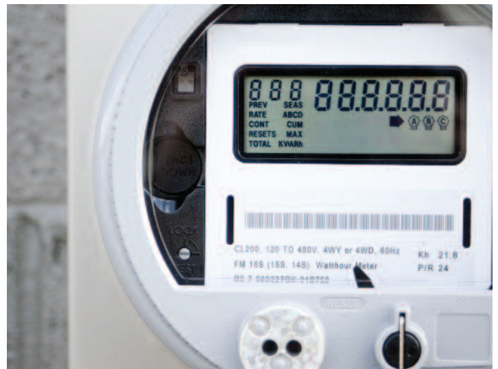
Figure 1: A new generation of gas, electricity and water metering products will be expected to report their readings regularly for billing and resource-management, while operating unattended for as long as two decades.
