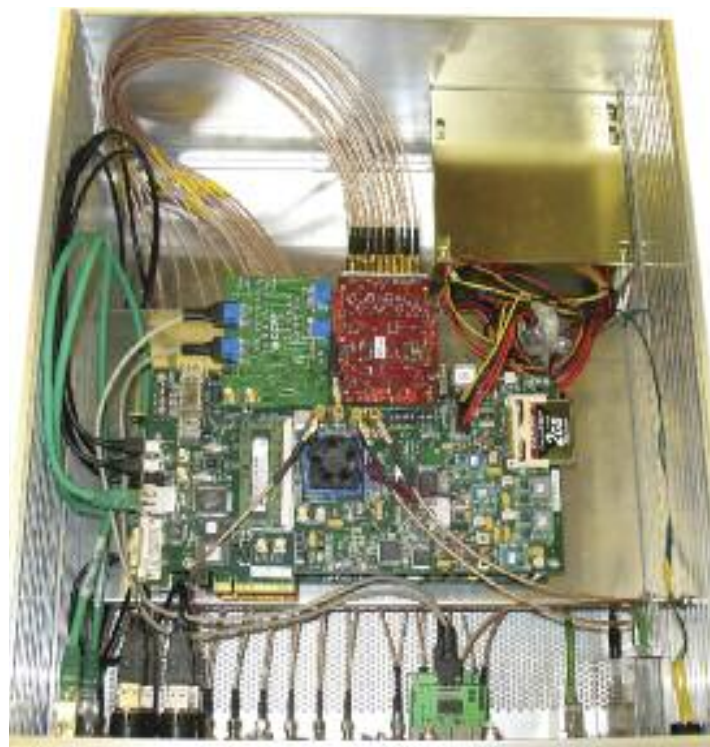
Figure 5: The FPGA data acquisition box comprises Xilinx's ML605 evaluation board, 4DSP's FMC108 ADC board and our in-house FMC/PMOD header board. We wired the ADC SSMC connectors internally to front-panel SMA bulkheads to extend the life of the ADC analog connections.
