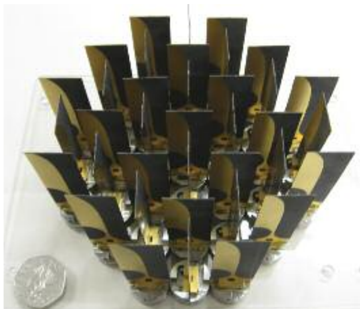
Figure 2: The microwave-imaging phased antenna array utilizes novel PCB antennas.
